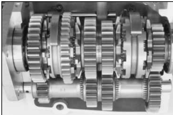
Light, But Legal - Y2K-4 transmission internals have a rotating mass lighter than any other NASCAR-legal transmission.
